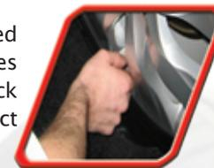
**STEP 2** Only measure pressure when your tires are cold. "Cold" means that your tires have been stationary for at least three hours or your car has not been driven more than 2 km.
