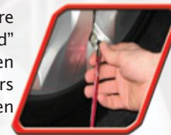
**STEP 3** Complete tire inflation pressure measurement: Remove cap from valve on one tire, press tire gauge onto valve and take pressure reading.
