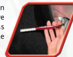
**Add Air** to achieve recommended air pressure. If you overfill the tire, release air by pushing on the metal stem in the center of the valve, then re-check the pressure.
