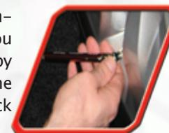
**Replace** the valve cap and repeat with each tire, including the spare.
